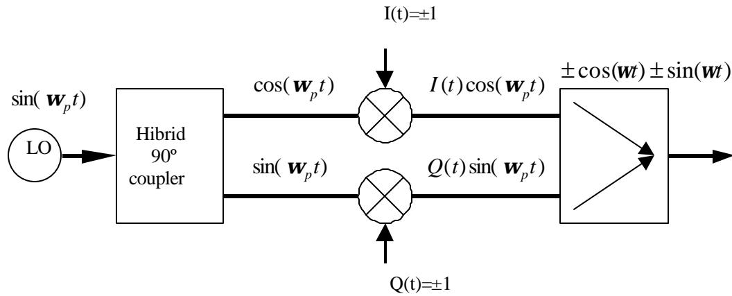
Fig. 1 Mixer Based QPSK Modulator
