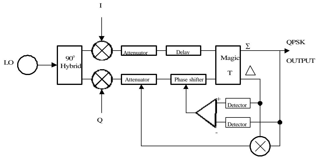
Fig. 2 Closed Loop Error Correction Mixer Based QPSK Modulator
